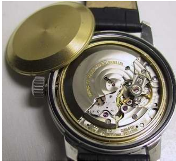
Cal. 8541B with its soft iron inner casing.
